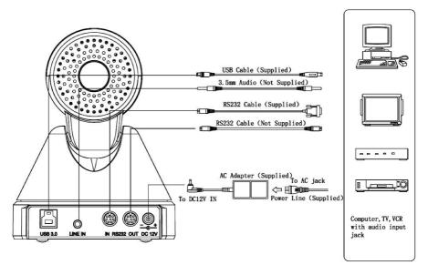
Step2. Power connected to the Camera, the front panel power lamp light.
