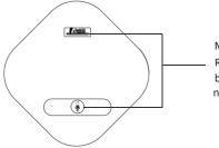
Microphone Status indicator RED: Microphone mute blue: Microphone working normally
